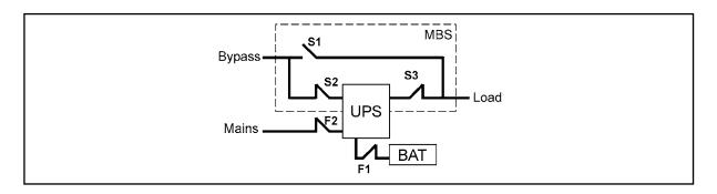
Figure 16 The normal positions of the three MBS switches.
